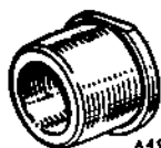
18G 123 AD. Camshaft Liner Reamer Pilot—Rear.
