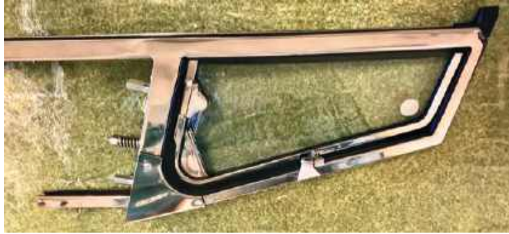
MGB quarter light unit showing support leg
