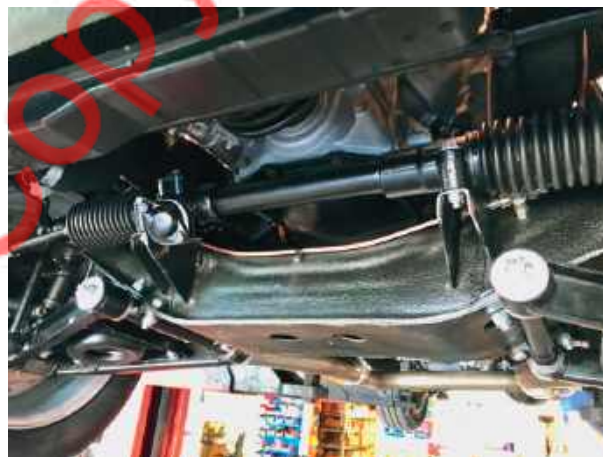
Front cross member showing steering rack and lower spring pans
