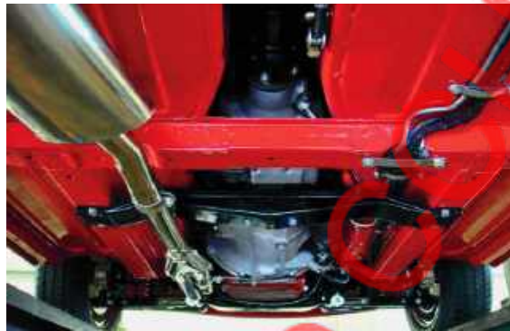
CCHL 5 Speed gearbox in an MGB
