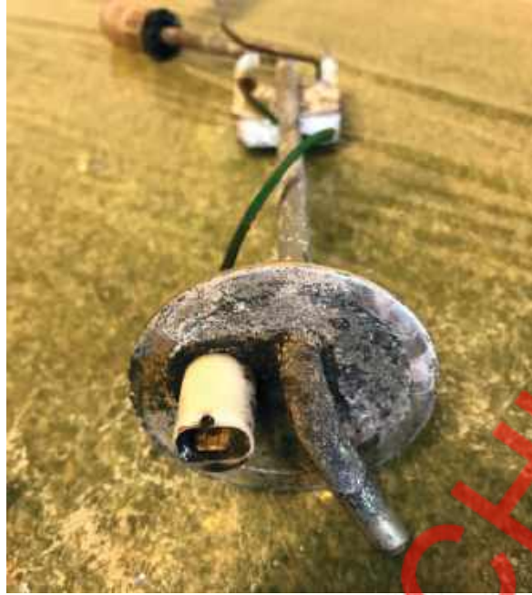
Tank sender unit for cars 1977-1980
