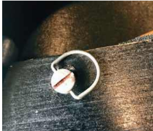
Example of a Dzus fastener
